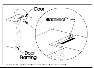
glazing seal in frame assemblies utilizing fire rated glass in both doors and side lites.
